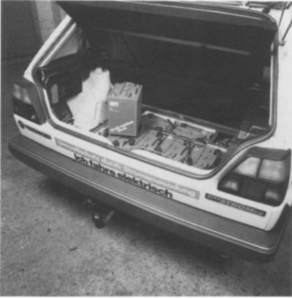
Fig. 8. Dryfit-battery installation in the trunk of the CityStromer by Volkswagen – Rhein. Westf. Elektrizitätswerke, Essen.
